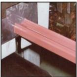
**Gesso**After the profile shape is milled, several layers of gesso primer are extruded over the wood profile to create a smooth surface.
